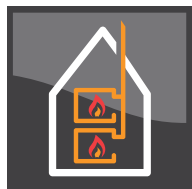
Decentralized multiple fireplaces connected to same chimney
